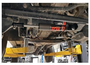
Fig. 2: Install the ATS stabilizer.
