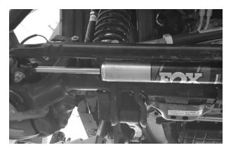
Fig. 5: Sufficient shaft clearance.
