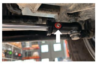
Fig. 3: Adjuster screw on eyelet.
