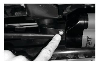
Fig. 6: Pinch bolt to rotate reservoir.
