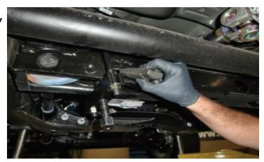
Push the torsion bar forward through the factory keyway cross member and lower control arm. You may need to use a hammer and punch on the end of the bar to break it loose from the keyway and control arm.
