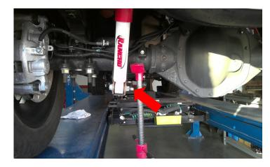
Loosen but do not remove the U-bolts on the passenger side. Remove the U-bolts completely from the driver side.
