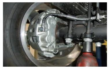
Lower the axle down enough to install the ReadyLIFT block on the driver side.
