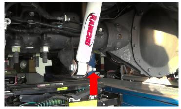
Reattach the brake line bracket to the axle. Use factory hardware torque to 5ft-lbs.
