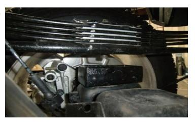
Raise the axle with the ReadyLIFT block installed to the leaf pack. Install the provided U-bolts and hardware. Only snug the U-bolts up enough to hold the axle in place. Repeat all steps on the passenger side. Final torque will be done when the vehicle is on the ground.
