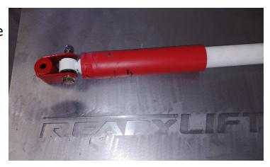
Reattach the shock to the frame using factory hardware. Hand tighten only, final torque will be done when the vehicle is on the ground.
