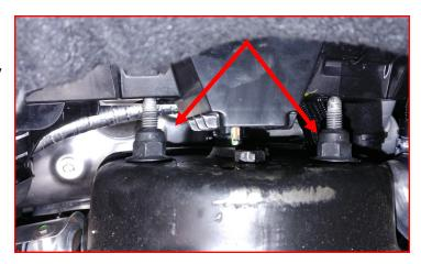
Remove the upper control arm bolts located inside the strut tower. Remove upper the control arm from the vehicle at this time. Discard the control arms.
