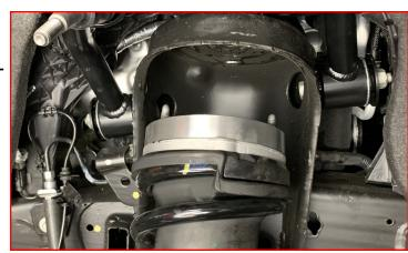
Install the factory lower strut bolts.
