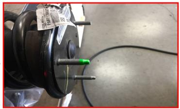
Using a 27/64" drill, drill 2 of the 3 upper strut mounting holes referenced in the picture to provide clearance for the upper studs. Passenger side is shown. The 3rd hole does not need to be drilled out. Be careful of wiring above the hole, move if necessary.
