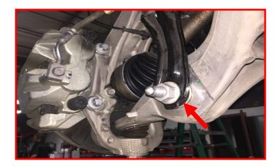
Separate the inboard axle joint from the differential and remove the axle from the vehicle.
