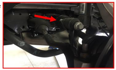
Remove the ABS sensor from the back of the hub. Remove the brake caliper bracket and support using a suitable hanger to prevent straining the rubber brake hose. CAUTION: Do not hang the brake caliper from the rubber brake hose.
