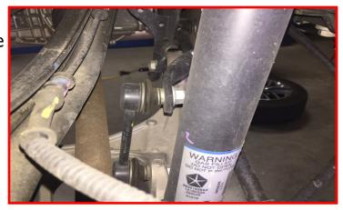
Loosen the 2 rear-most control arm bolts at the cradle, and disconnect all 3 control arms at the knuckle.
