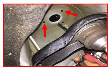
Locate the ReadyLIFT front strut extension. Passenger side shown. Install to the top of the strut using the factory hardware. Torque to 30 ft-lbs.
