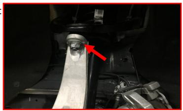
Remove the lower strut hardware.
