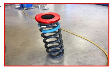
Install the spring and spacer assembly and raise the lower control arm to connect the upper control arms. Do not tighten at this time.
