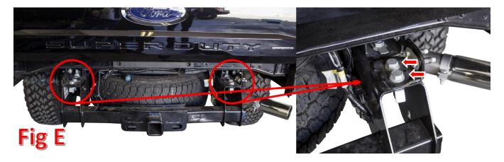
6. Remove the parking sensors from their outer rings. Do this by spreading the two tabs on the back side of the outer mounting ring, then pushing the parking sensor out the back of the outer mounting ring. Leave the sensors plugged into the rear bumper wiring harness. Make sure to keep track of where each sensor was mounted to your OEM bumper. You have to mount them to your new bumper in the same order. (Fig F)
