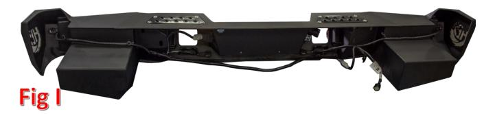
6. Mount the supplied ADD Bumper Mounting Brackets. Use the bolts you saved from Removal Step 5, but install them upside down from the way they were originally installed. Then, use the supplied 1/2" Bolts (x4), 1/2" Washers (x8), and 1/2" Nuts (x4) on the remaining mounting holes with the bolt heads facing outwards. Refer to Fig J. Once all bolts have been loosely installed, torque the OEM bolts to OEM torque specification, and torque the supplied 1/2" Bolts to 70 foot pounds.
