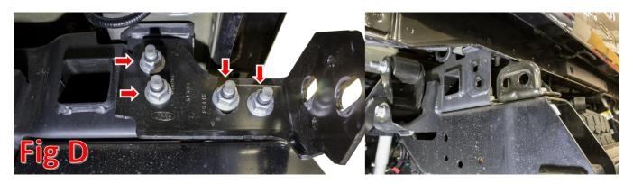
5. Remove the OEM Frame Rail Bracket. Use a 15/16" Socket to remove the two mounting bolts (per side), then remove the bracket. Save these bolts for reuse. (Fig E)
