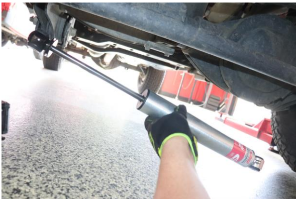
Step 5. Install the Eibach steering damper in the truck with the body of the damper facing the driver's side of the truck.
