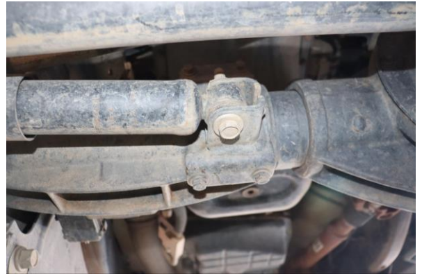
Step 2. Remove 18mm bolt from driver side of OE damper at the axle.
