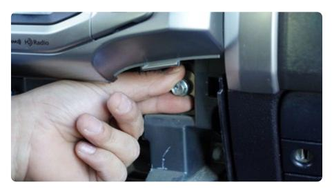
STEP 8 | Install the control cluster and dash trim by applying pressure until the clips are secured.
