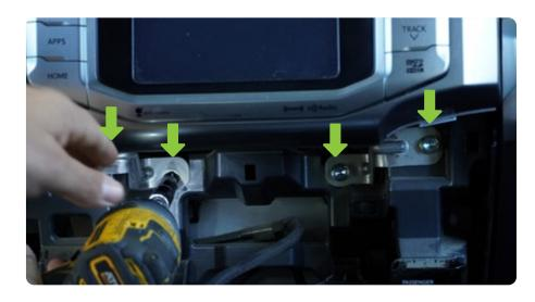
STEP 5 | Drill out the marked holes using an 11/32" drill bit.
