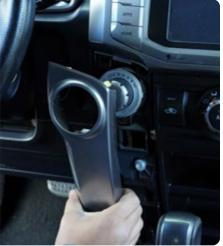
STEP 2 | Remove the control cluster by pulling towards the rear of the vehicle to release the clips, and disconnect the wiring connector on the back.
