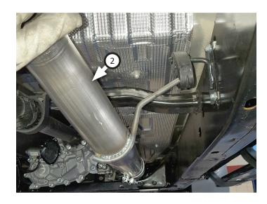
Place clamp (7) onto muffler (3) then connect it to intermediate pipe. Tighten clamp just enough to allow for adjustment then place clamp (7) onto muffler outlet.
