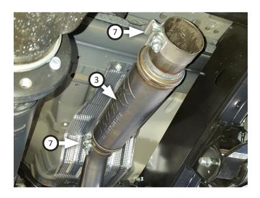
10. Route **tailpipe (4)** over axle and connect it to muffler. Insert wire hangers into isolators and tighten clamp just enough to allow for adjustment.
