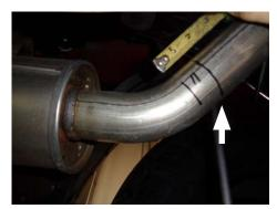
4. Cut driver and passenger side tailpipes off at marked lines and remove them from vehicle.
