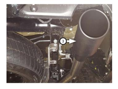
9. Place **tip (3)** onto left tailpipe. Tighten inlet to secure connection.
