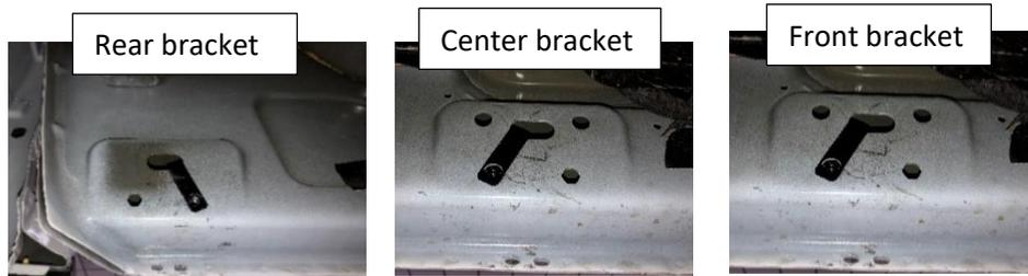
U-clip positioning. **NOTE:** U- Clip orientation will be the same for passenger
