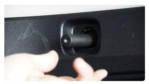
STEP 7 | Begin installing molle panel by securing it to the factory mounting location above the rear window using the factory bolt and a 10mm socket.
