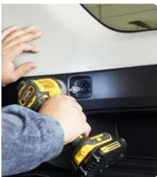
STEP 5 | Remove the plastic tie down next to the rear lift gate door by turning it to unlock, and pulling it out.
