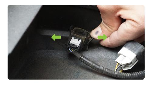
**STEP 7** Use needle nose pliers to squeeze the release tabs and push up from underneath the bumper, and have a friend pull up on the trim from the top of the bumper.
