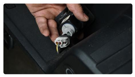
**STEP 5** | Press the release tab on the smaller plug and pull to remove.
