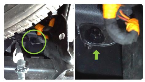
STEP 26 | Connect the bumper wiring harness plug to the vehicle wiring harness by pressing it into the connector and rotating the lock into place.
