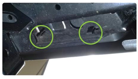
**STEP 8** Disconnect the plug for the sensor wiring harness located between the driver side frame rail and the spare tire by rotating the lock-release and pulling.
