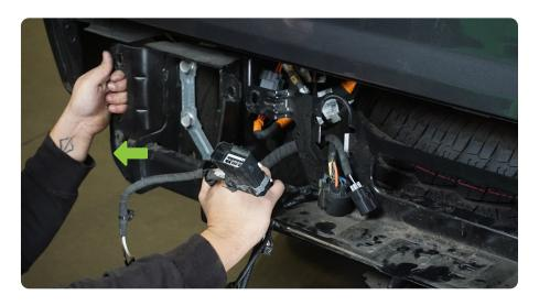
**STEP 13** | Remove the lock for the spare tire by rotating the lock and pulling out.
