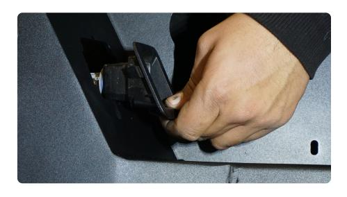
STEP 16 | Install the trailer plug on the DV8 bumper by pressing it until it "clips" into place.
