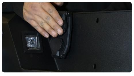
STEP 17 | Install the license plate using the provided M6 hardware with a 4mm allen bit and 10mm socket.
