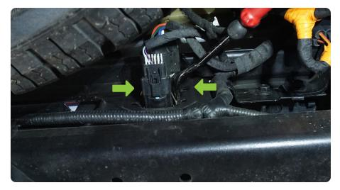
**STEP 3** Remove the trailer wiring plug from the bumper using a trim clip tool to press in the release tabs on both sides of the plug and push it out of the bumper.
