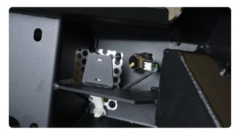
**STEP 24** | Connect the trailer wiring harness and plugs by pressing them until they "clip" into place.
