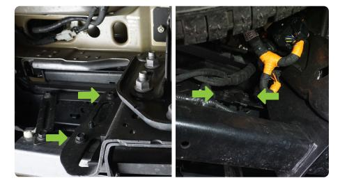
**STEP 11** Use a trim clip tool to remove the clips securing the sensor wiring harness to the bumper.
