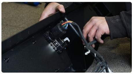
**STEP 25** | The small section must be removed to accomodate the DV8 bumper.
