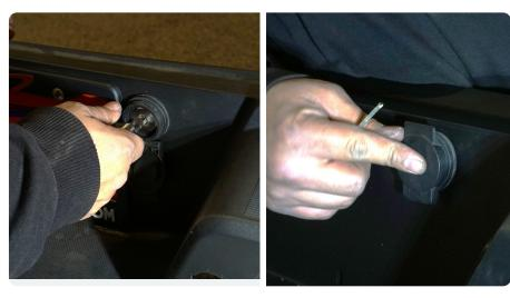
STEP 14 | Use a trim clip tool to remove the sensor bezels from the factory bumper by pressing the small tabs securing the bezels and pushing them "out" towards the front of the bumper.
