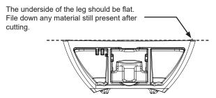
To fit legs to pioneer trays, QMPS10 must be purchased as separate. Install the spacer kit as shown.
