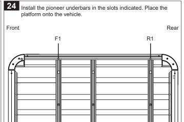
Once Pioneer underbars have been aligned properly over the channel nuts on the legs, tighten all hardware using the allen key provided. Ensure channel nut has rotated within Pioneer underbar and is fixing Pioneer securely.
