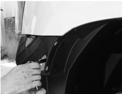
**Figure 6 - Support Bracket Removal**
