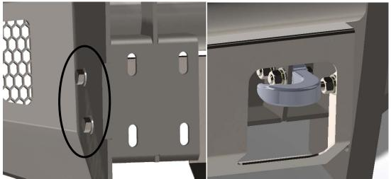
Figure 10a (bolt location for lower guard)
