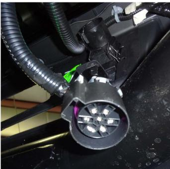
Figure 3a (ELECTRICAL HARNESS DISCONNECTED)
