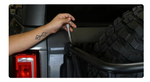
STEP 12 | Install the provided M8x75 hardware next to the pin using a 5mm allen bit and secure. This will help to prevent any up and down movement of the carrier in the latch area.
