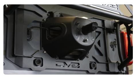
STEP 6 | Secure the tire guard to the hinge using the provided M8x50mm hardware with a 5mm allen bit.
