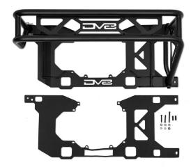
STEP 1 | Lay the tire guard on a soft surface to prevent damage to the product and apply the provided foam to the tire guard where it will contact the vehicle starting on the hinge side.
